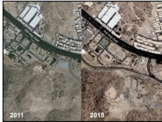
Fig.(3): Satellite images acquired in 2011 and 2018 showing the locations of rock cutting and land filling activities to the northeast of Gabal Thawr.
