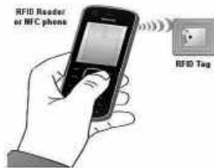
Fig. 4: Communication between mobile phone and RFID/NFC tags.
