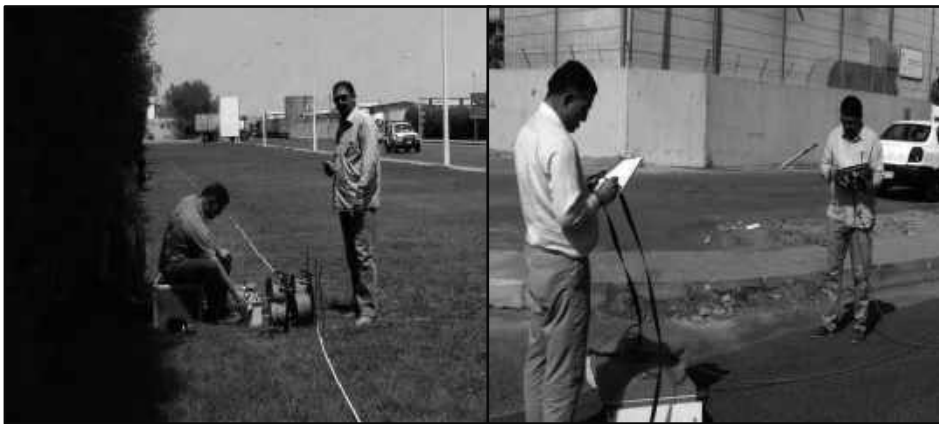
Fig. (5): Field measurements of VES's and GPR profiles in the 1 st industrial zone, Jeddah.
