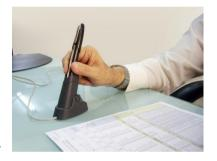
The Pen camera codes the stroke location into the memory, after transferring this data to the server the data is decoded to recreate the stroke on a similar e copy of the paper used to write on; by doing so the e-restructure e form looks like a scan of the original paper.
