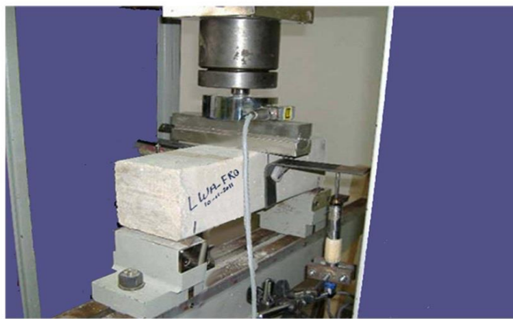
(c) Test set-up in 1000 kN testing machine
