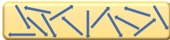
Figure 1.9: Schematic diagram illustrates the diamagnetic materials.
