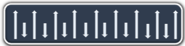
Figure 1.13: Schematic diagram illustrates the ferrimagnetic materials.
