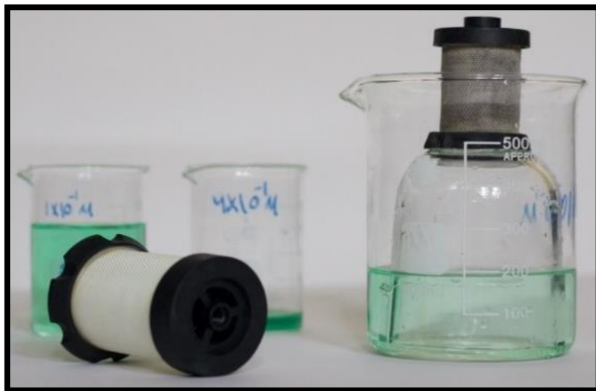
Figure 4.21: Illustration image of filter element including nano samples (AuNPs, AgNPs, FeNPs, or CoNPs).
