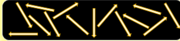
Figure 1.10: Schematic diagram illustrates the paramagnetic materials.
