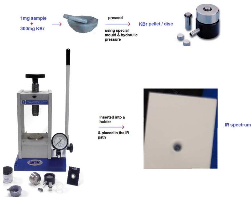
Figure 3. 38: The preparation of a KBr for IR spectroscopy.
