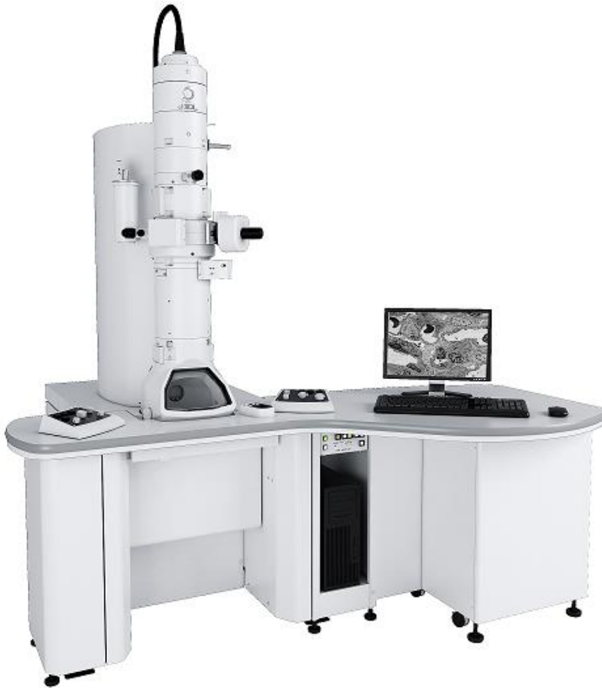
Figure 3. 22: JEOL Transmission Electron Microscope model (JEM – 1400) with LaB 6 cathode, the maximum voltage is 120 kV, the resolution is 0.2 nm, and the maximum magnification is 1200000X.
