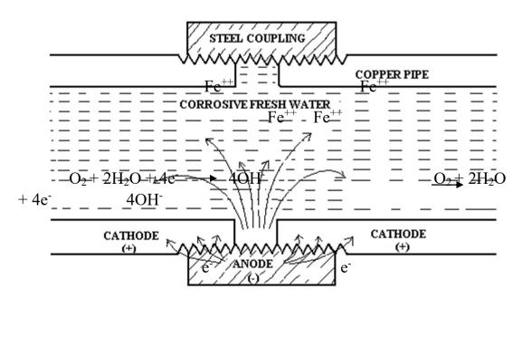
Fig.(1.1): The basic corrosion cell consists of an anode, a cathode, an electrolyte, and a metallic path for electron flow. Note that the corrosion current (i) enters the electrolyte at the anode and flows to the cathode.
