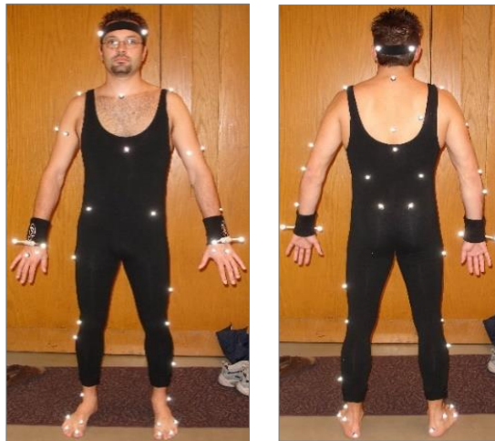
Figure 1.5: Marker-based MOCAP. An actor wearing a motion-capturing suite with a set of markers attached to his body (Carnegie Mellon University - motion capture library - info).
